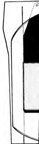
Cut-away side-view of a pad in safety-pants. Note the sleeve in the knee area and snaps on top.
