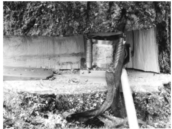
Pictured Above: A tree jack in its seat on a nice second growth tree. A few pumps on the handle and this tree fell right where it was supposed to.
