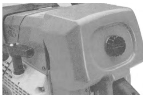
A Max Flow filter system with the rain-cover.
